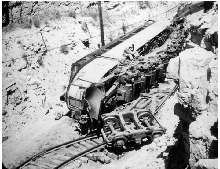
The lead engine, E78, on its side in the cut almost half-way through the curve.
